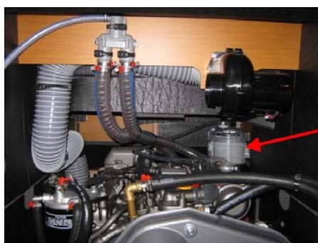
Sea water filter Location: Engine compartment
