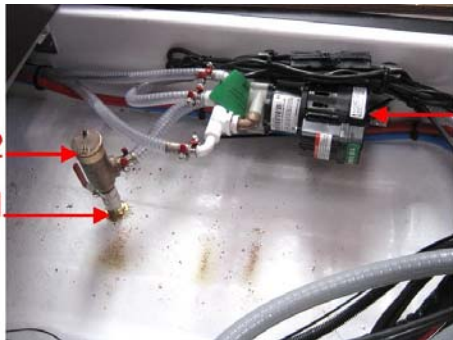
Seawater suction strainer for engine
