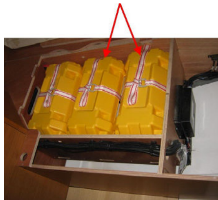
Spare service batteries: 2 x 115A
