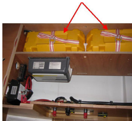
Spare service batteries: 2 x 115A
