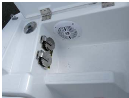
Ref 2: Shore power socket (Air conditioning / House)
