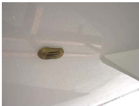
Seawater suction strainer for engine
