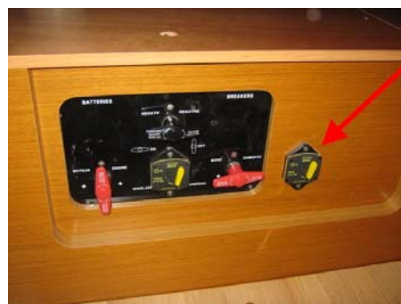
Breaker - 30A Location: Starboard aft cabin
